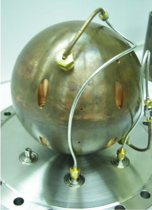
Schematic of a quasi-spherical resonator: a 'race-track' cavity.
